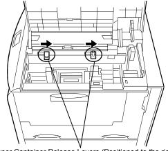
Toner Container Release Levers (Positioned to the right)
